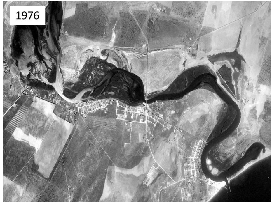
Figure 4.4. Historical photographs of the Berg River Estuary mouth, in 1942 (with the natural mouth) and in 1976 (after canalisation and construction of the artificial mouth). Note the new, permanent mouth and 'blind arm' parallel to the coast in the 1976 image (Beck & Basson, 2007).
