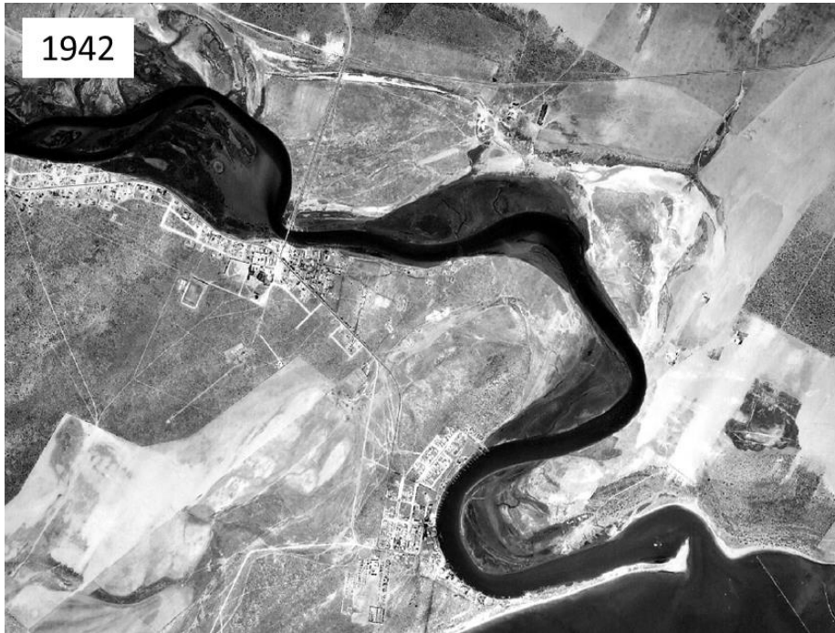
Figure 4.4. Historical photographs of the Berg River Estuary mouth, in 1942 (with the natural mouth) and in 1976 (after canalisation and construction of the artificial mouth). Note the new, permanent mouth and 'blind arm' parallel to the coast in the 1976 image (Beck & Basson, 2007).
