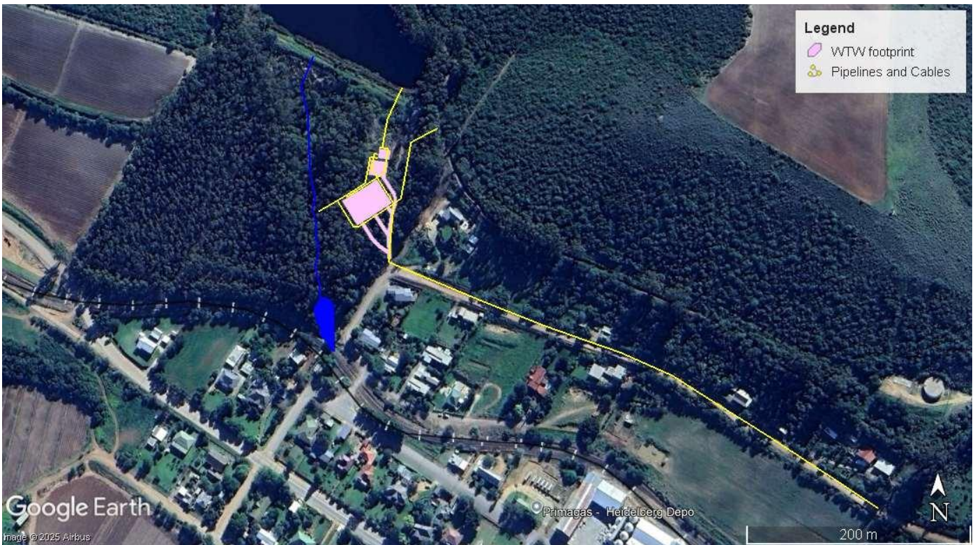
Figure 6: Map showing the proposed development in relation to a confirmed watercourse shown as a blue line and polygon (wetland) as delineated by Enviro-EAP. Note the proximity of the proposed WTW to the watercourse.
