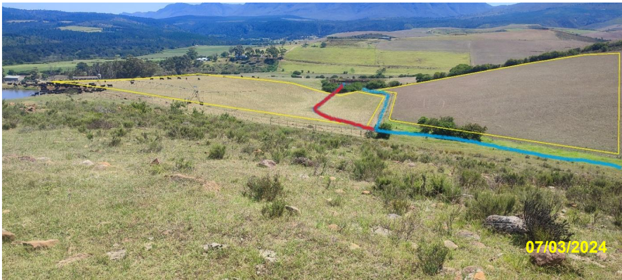
Site Photo 5: Proposed prospecting areas on transformed cultivated land and transformed drainage line east of regional road on Farm Wegwyzersrivier RE/582. Red line indicates where drainage line was historically located, blue line indicates route along which drainage line is currently channelled. Channelled drainage line and original drainage line route not to be prospected upon.
