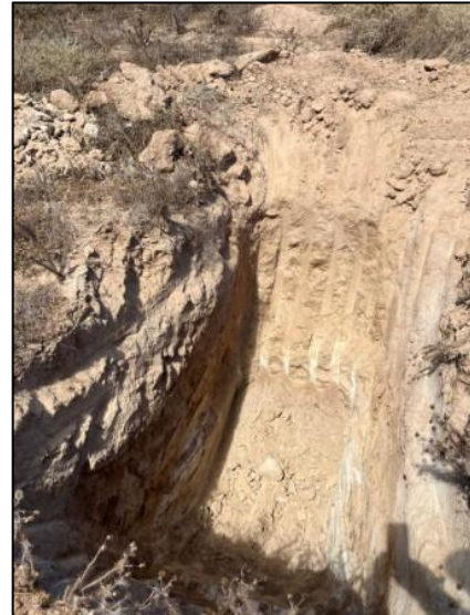
Plates 9 & 10: Test pits mostly refused at relatively shallow depths on the very dense dorbank, in some areas beneath the site
